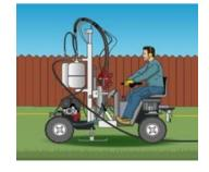
garden. These holes will then have compressed air blasted into them causing a network of fissures, which create a comprehensive drainage network. This improves natural drainage throughout the Square and enhances soil composition. The process is environmentally friendly as it limits excess water draining into local drainage systems. Click the link to see the machine in action <u>Terrain Aeration</u>
